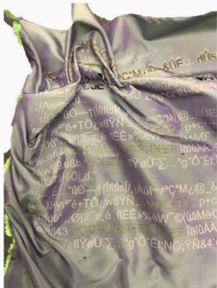
laser cut (engraved) coding on to reflective silk taffeta, with attempts of arrow smocking
