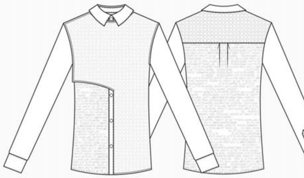
top layer with grid laser cut; bottom layer with coding engraving; separate center placket pattern with the bodices piece sandwiched in
